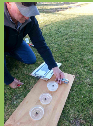
4: Using a timer leave the sample for 10 mins. Then observe how much the dispersion has occurred at the 10 min mark.
