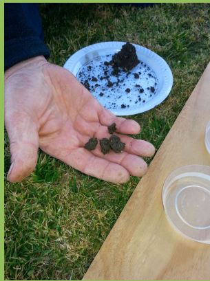
2: Get a small 3-5mm aggregate from 10cm depth that has been air dried for 24-48 hrs.
