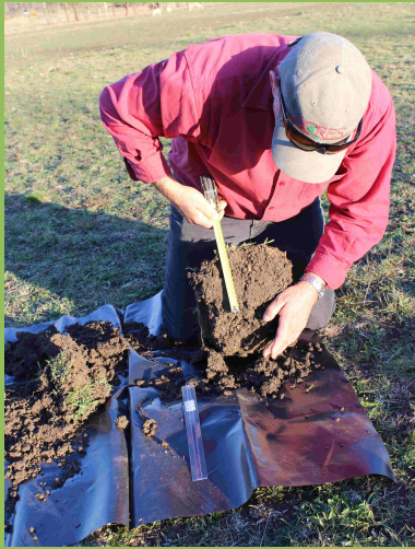
Step 2: Place the cube on its side on a sheet and carefully count the roots at 20cm.
